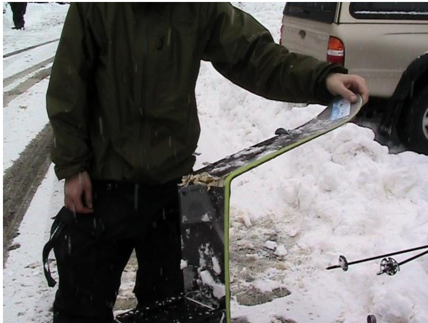
Splitboard broken by impact with a tree during a snowboarder triggered avalanche on Becker Peak, Echo Summit, CA. Two snowboarders caught, 1 partially buried. Photo: Kelley Rogers.
