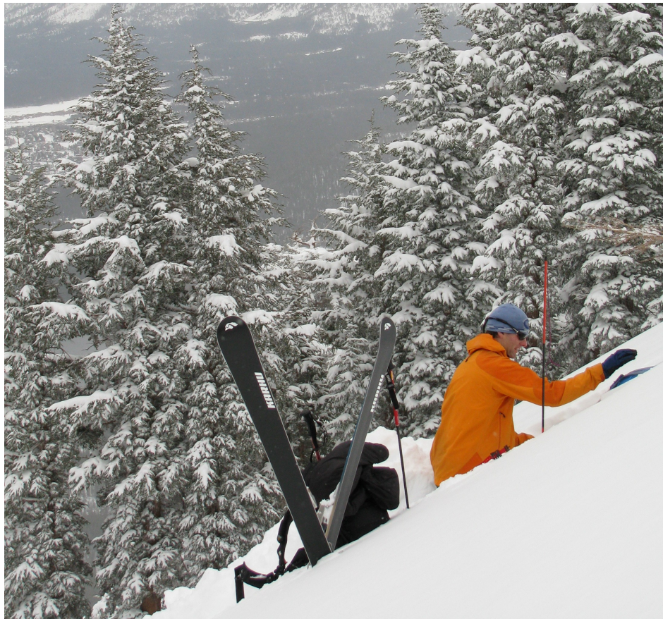
Forecaster Brandon Schwartz performing layer bonding tests in the pit. Mt. Tallac, CA
